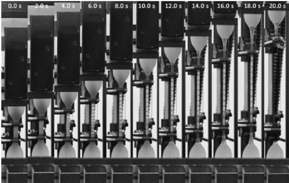
Figure 4.10 – SG tensile test at 500 mm/min time lapse, all shots<sup>11</sup>
