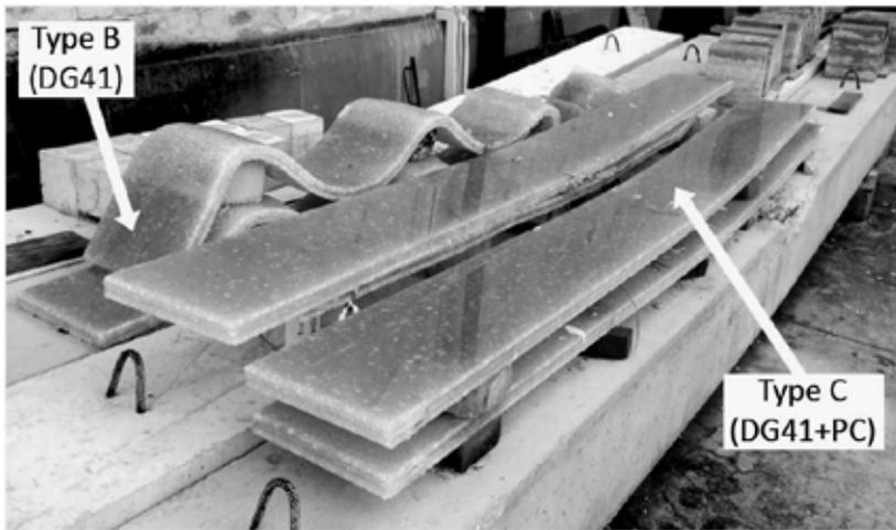
Figure 4.62 - long-term weathering effects on FDLG
