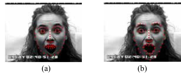
Fig. 3. Matching between a facial model and an image. (a) shows the initialization and (b) the fitted model.
