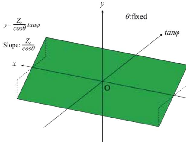
Fig. 8 Ray-space in  $(x, y, \tan\varphi)$  space with fixed  $\theta$  captured by linear arrangement cameras.
