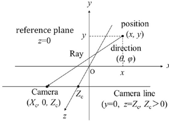
Fig. 6 Ray capture by linear arrangement cameras
