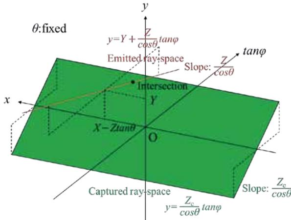
Fig. 10 Captured ray-space, emitted ray-space and their intersection in  $(x, y, \varphi)$  space with fixed  $\theta$ .
