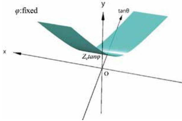
Fig. 7 Ray-space in  $(x, y, \tan\theta)$  space with fixed  $\varphi$  captured by linear arrangement cameras.
