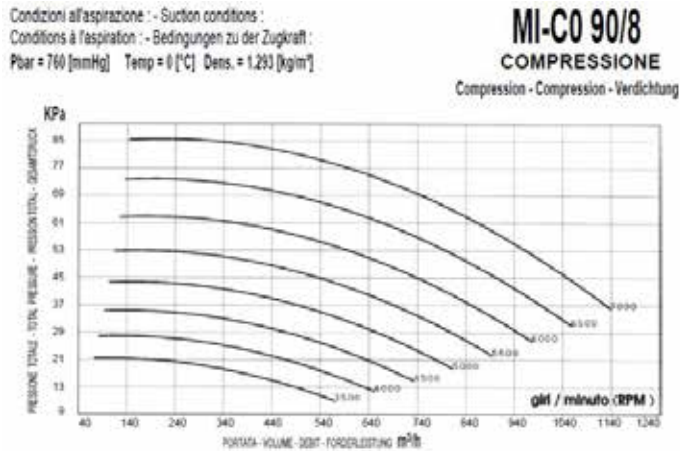
Fig. 3. 18 Centrifugal compressor performance curves
