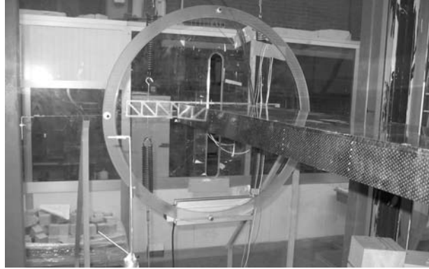
Figure 8.1 Rectangular section: wind tunnel model with pressure taps
