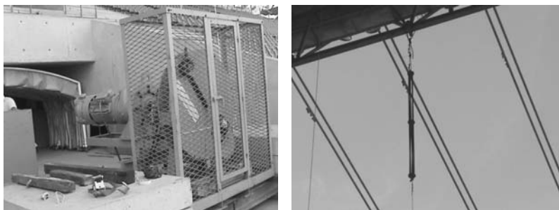
Figure 4.27 View of the electric engine with the eccentric link (left) and of the girder linked spring (right).
