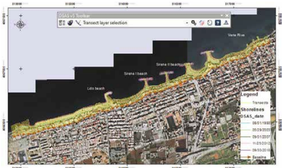
Figure 10 - Digitizing of the shoreline and the baseline as well as the realization of the transects using the DSASv5 tool.
