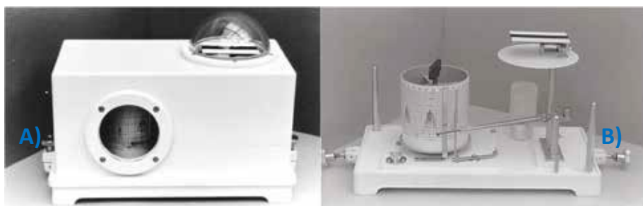
Figure 6 - Robitzsch's bimetallic pyranograph (1932): external view (A) and internal view (B). Photo by G. Fasano.
