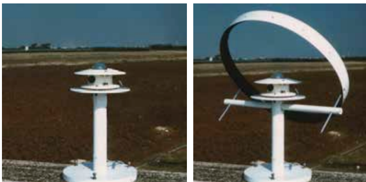
Figure 7 - Current version of pyranometer (Eppley model PSP, 1957): on left for global radiation; on the right the same instrument equipped with a shading band for the measure of diffuse radiation.
