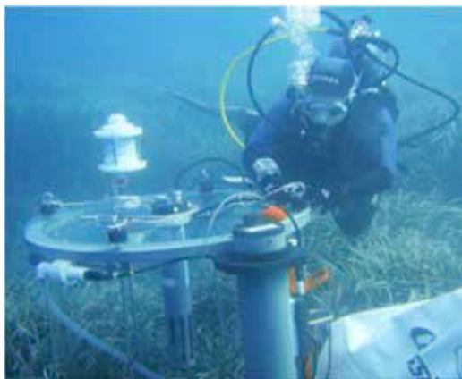
Figure 9 - SuMaRad and Benthic Chamber, during the installation phase on the seabottom of Cavo (Elba Island-Italy). Photos by Gianni Fasano.
