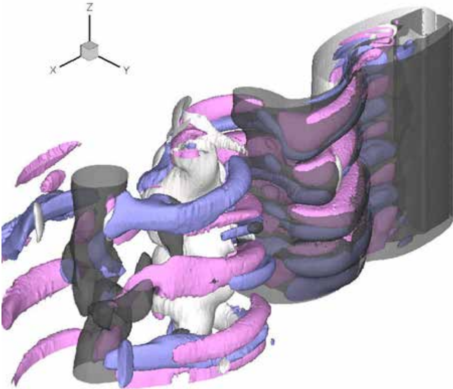
Figure 8: Isosurfaces of the streamwise and spanwise vorticity components in the wake obtained at Re = 300 after the transient. The black and light gray surfaces correspond to \omega_z = -0.4 and \omega_z = 0.4 respectively. The pink and blue surfaces identify \omega_x = 0.4 and \omega_x = -0.4 respectively.
