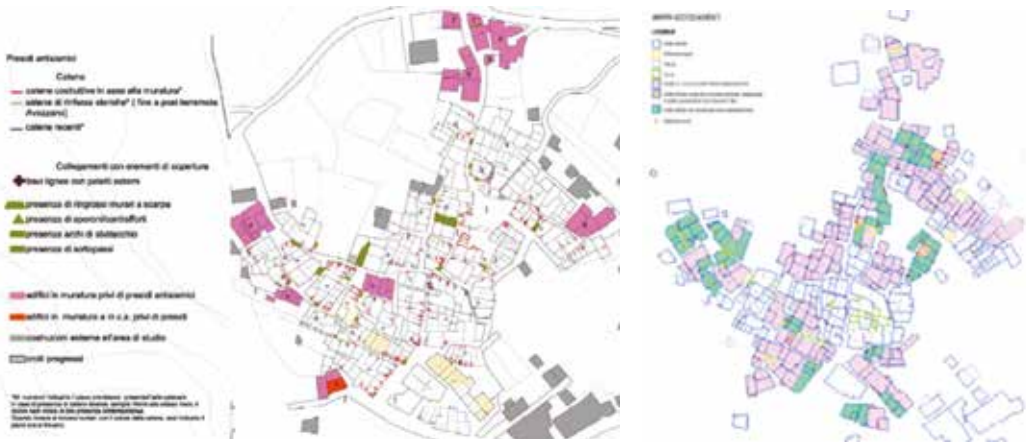
Figs. 2a - 2b Left: Thematic map relating to the presence of anti-seismic devices. Right: Thematic map relating to the study of the different evolutionary phases of the aggregates (source: Carocci et al. 2010) Amatrice (RI). (Veronese, 2019).
