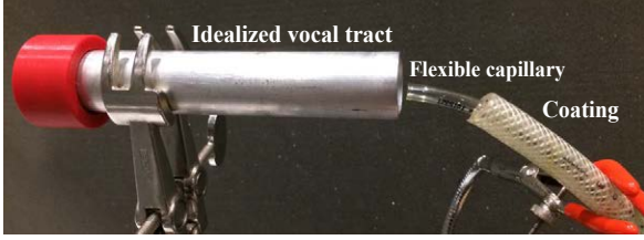
Figure 1 – Photo of excitation at the waveguide inlet.
